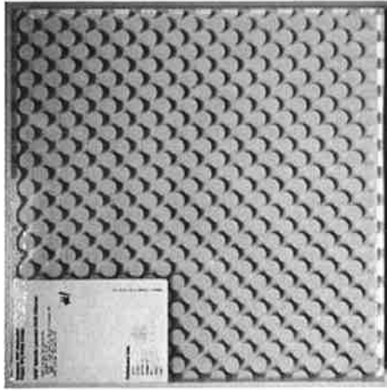
FRITTED GLASS AT ROOFS main span
