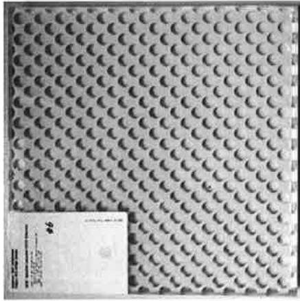
FRITTED GLASS elevator shaft walls
